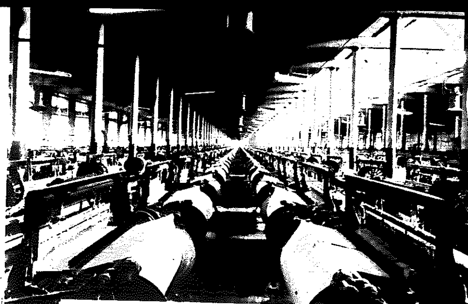
Textile Mill, and plenty of it: Weave room of the Lancaster, S. C., plant of the Springs Cotton Mills. One of the largest print cloth weave rooms in the world. Seven thousand looms in this one building turn out more than a thousand miles of cloth a week.
