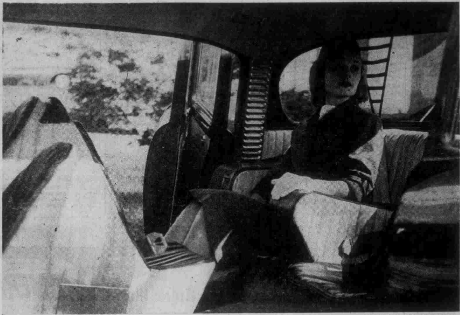
Unique automobile packages passengers as well as science and design can do it. Padded bucket seat surrounds most of the body as a bar against sudden lurch. Nylon harness behind head protects against "whiplash" of crash from rear. Note the absence of projecting knobs.
